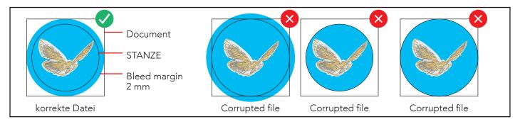
The file must always be saved in PDF format and besides the graphic must also include a 0.1 mm or 0.283 pt. die cutting contour (also with simple geometric shapes like rectangles or circles).
